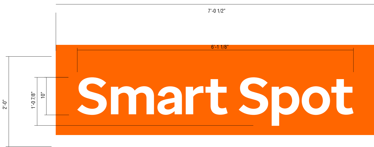
4a 1 INTERIOR FCO LETTER ON BACKGROUND LAYOUT - 10" SCALE: 1" = 1' - 0"
